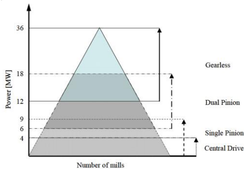
Fig 7.1 Typical mechanical mill configurations [4]
