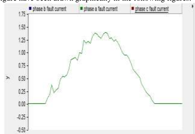
Characteristics of fault current phase-A.
