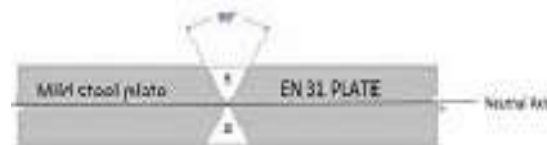
Fig. 3: V-Groove Schematic geometry
