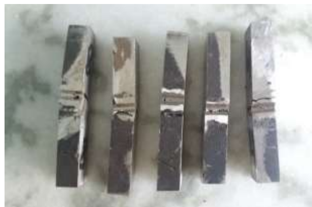
Fig.7: Specimens for Impact Toughness
