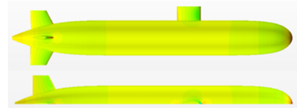
Fig.7. Streamline and flow rate along the hull at speed V=3.05\text{m/s}
