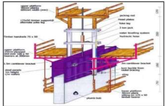
Fig 4 :- Components of Slip Formwork
