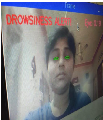
Fig.11. Drowsy detection using EAR ratio
