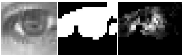
Figure 3: Left to right: A blurred eye image; the areas considered dark enough to be pupil candidates; our estimates of centre probability in the regions that were dark (white=highest probability). Note the spurious peak on the left.
