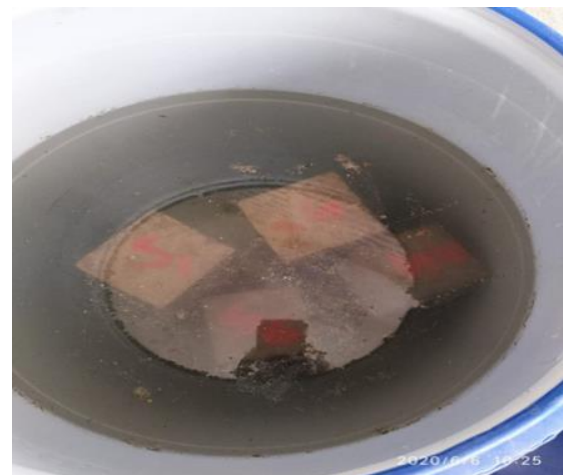
Figure.3 Cubes cured in Acid
