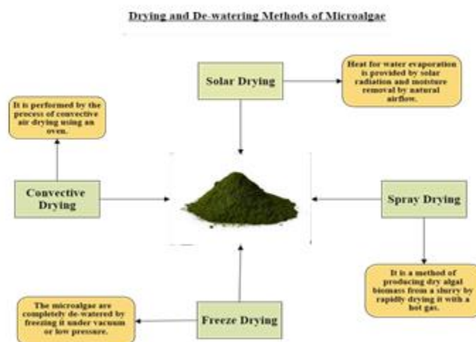
Fig. 6 – Drying and dewatering methods of microalgae
