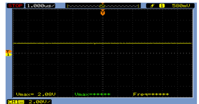
Fig. 27. Output voltage in step-down mode
