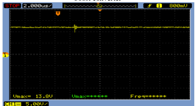
Fig. 26. Output voltage in step-up mode
