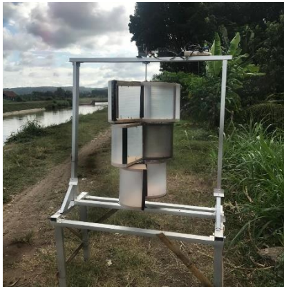
Fig. 13. Multi-level Savonius Wind Turbine with Fixed Rotational Axis
