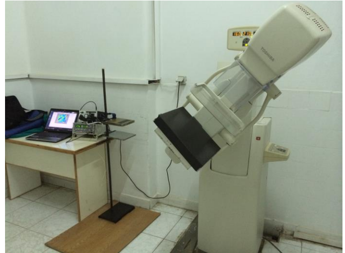
Fig. 3. X-ray Mammographic machine in adjacent to EBT system
