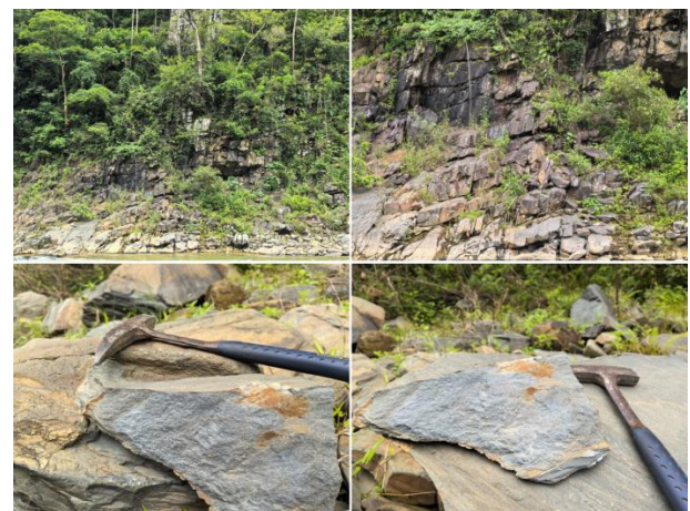
Fig. 3. Typical outcrops and textures of quartzitic sandstone found in the project area
