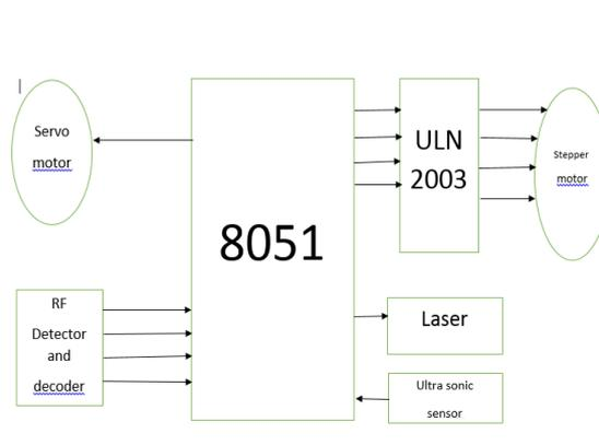
By using ultrasonic waves we can detect the missile then micro controller activate the laser. This mechanism is kept such that the servomotor is attached with the ultrasonic sensor while it is kept above the stepper motor. Additionally we have kept the provision of friendly plane safety by using RF module so that it identifies that the object is hostile or not.
