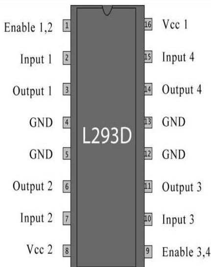
L293D is motor driver IC which is useful for rotating motor in clockwise and anticlockwise direction. It is a bidirectional IC. Also provide 12v supply to the motor.
