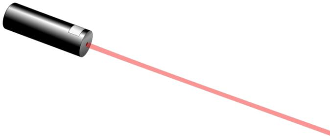
It is Light Amplification (by) Stimulated Emission (of) Radiation. Any device that emit highly amplified and coherent radiation of one or more discrete frequencies. LASER delivers light in an almost-perfectly parallel beam (collimated) that is very pure, approaching a single wavelength. Well basically it is used to produce a coherent non dispersing beam of light by multiple refractions inside a highly polished glass cavity.
