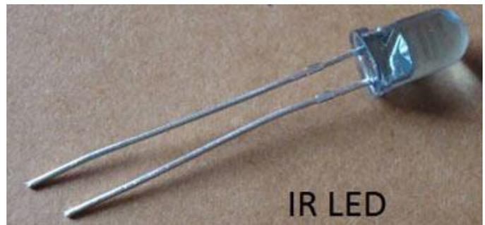
IR LED emits infrared light, means it emits light in the range of Infrared frequency. We cannot see Infrared light through our eyes, they are invisible to human eyes. The wavelength of Infrared (700nm – 1mm) is just beyond the normal visible light. Everything which produce heat, emits infrared like our human body. Infrared have the same properties as visible light, like it can be focused, reflected and polarised like visible light.
