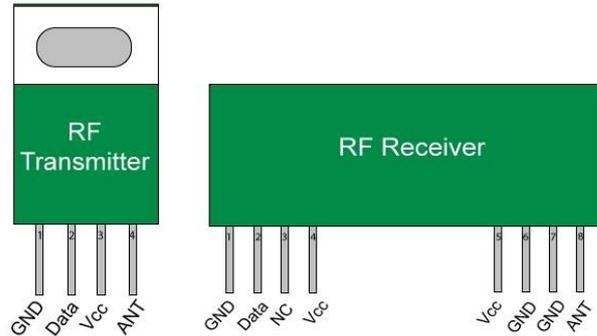
RF Transmitter is use for transmit the wireless data from input side. It operates at 434MHz frequency. for communication purpose we need serial data so we use Encoder HT12E, it converts parallel data into serial form at transmitter side. and at receiver side decoder HT12D converts that serial data in to parallel form.
