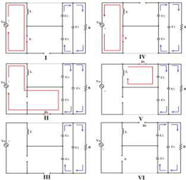
Fig. 6. Operating modes of DCM step-up rectifier
