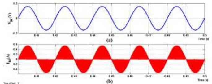
Fig. 7. (a) Input voltage, (b) Input current of parallel combination of boost and buck-boost converters
