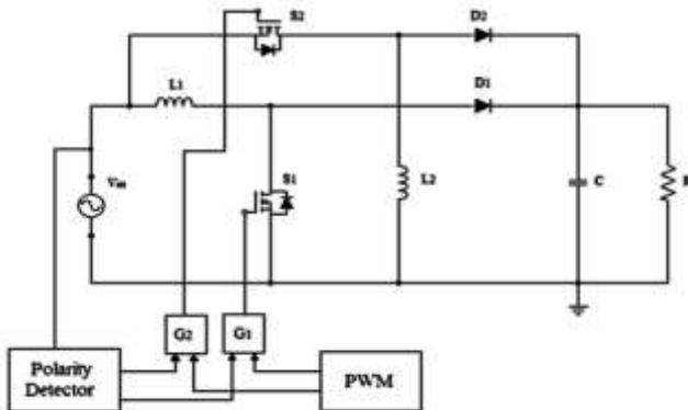
Fig. 1. Parallel combination of boost and buck-boost converters [6]
