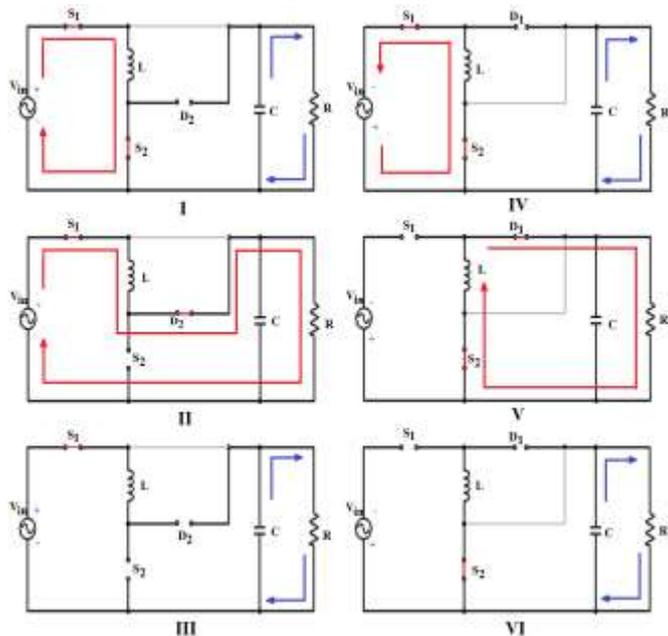
Fig. 4. Operating modes of bridgeless boost rectifier
