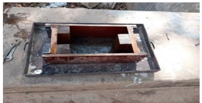
Fig. 4. Wooden Brick Mould
