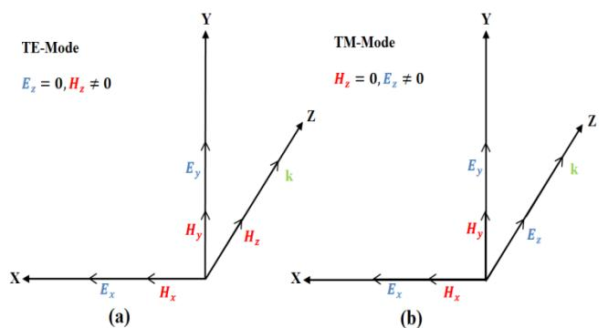
Fig.3. Components of EM fields in a rectangular waveguide: (a) TE mode  $E_z = 0$ , (b) TM mode  $H_z = 0$
