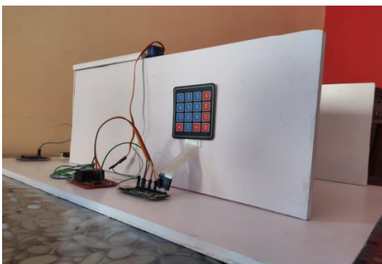
Fig 13: Door locking system using OTP
