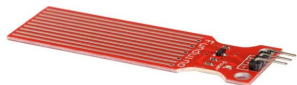
Figure 2: Water level Sensor
