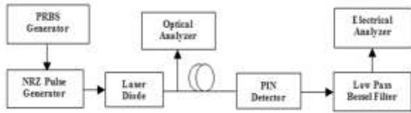
Fig. 1. Simulation setup for the single mode laser.
