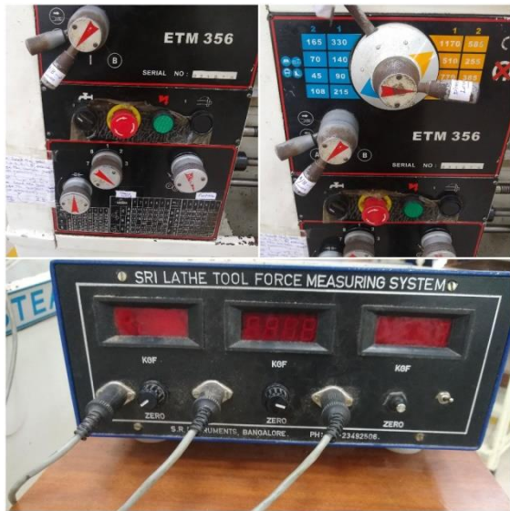
Figure 2: Lathe Machine And Machine-Tool Dynamometer
