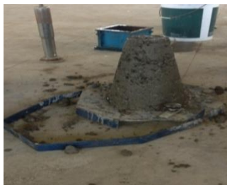
Fig 3 – Slump cone test
