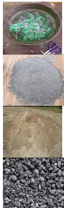
Fig 2 Plastic Cover, Cement, Sand and Gravel
