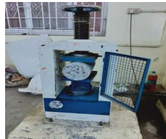
Fig 6 – Split tensile test
