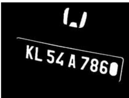
Fig. 4. Connected Components (Blobs)
