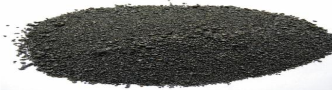
Fig. 1. Appearance of Copper Slag Sample
