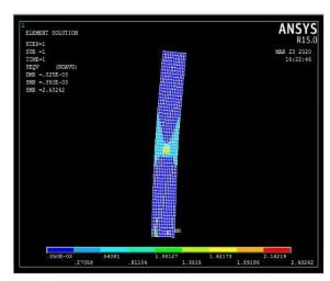
At 90°: The above figure shows the high wind pressure follow up on the aluminium mounting structure part. At 90 degree the part gets high wind power at the yellow locale and lower wind force at
