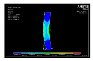
At 90° of rotation: The above figure shows the high wind stress act on the stainless-steel mounting structure part. At 90 degrees the part gets high wind force at the yellow region and lower wind force at the dark blue region.
