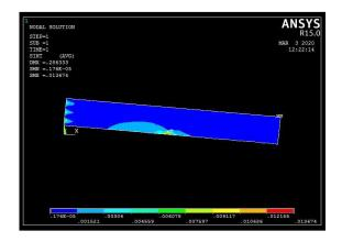
At 180°: The above figure shows the high wind stress act on the stainless-steel mounting structure part. At 180 degrees the part gets high wind force at the red region and lower wind force at the dark blue region.
