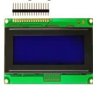
Fig 3:LCD Display
