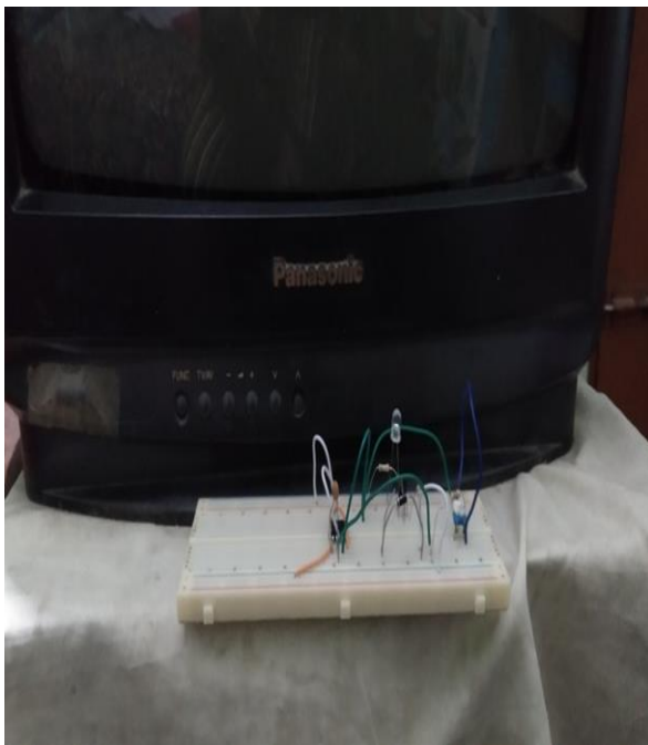
Fig. 11. The Tv remote jammer in front of TV before connecting power supply
