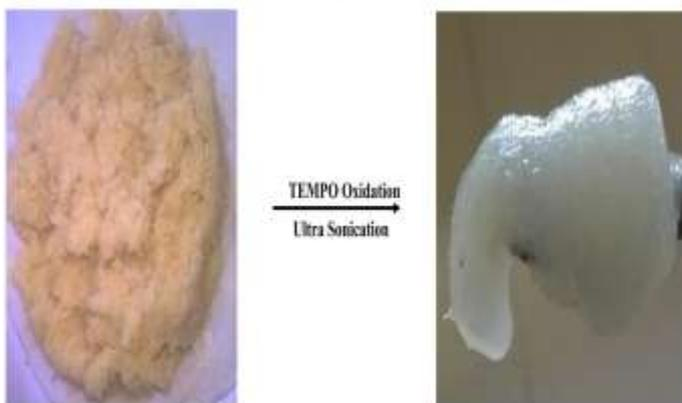
Figure 2: Digital images of preparation of TEMPO oxidized nano cellulose fibers from Micro fibrillated cellulose
