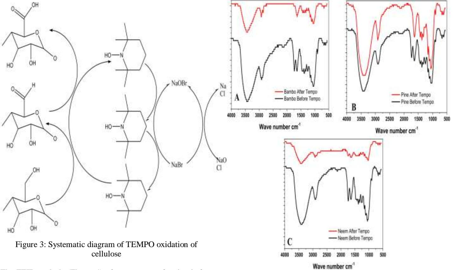
Figure 3: Systematic diagram of TEMPO oxidation of cellulose
