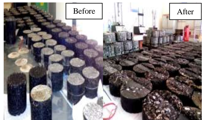
Fig. 10. Gyratory Samples Before and After Tests
