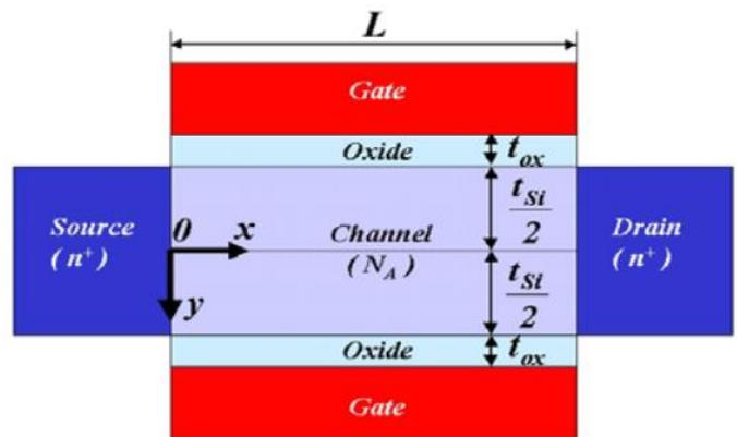
Fig. 1. Cross-section schematic of a DG MOSFET.
