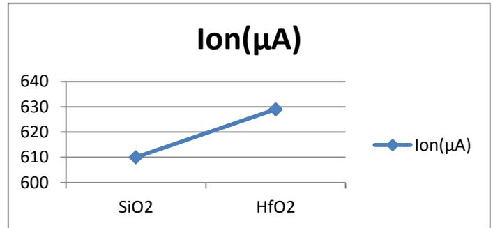
Fig.7. Variation in  $I_{on}$  with different dielectric DG-NMOS
