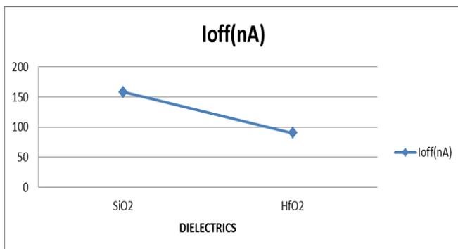
Fig. 6. Variation in  $I_{off}$  with different dielectric DG-NMOS
