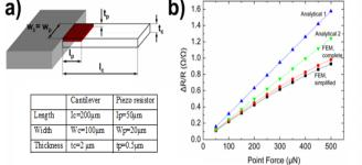
The deviation of FEM solutions from the linear behaviour is caused by geometric linearities at large tip deflections  $47.0\mu m$  at  $500\mu N$  is accounted in this type of analysis. The two FEM solutions differ by no more than 5.3% which indicates that stress difference is good. So the force sensing cantilevers should be made thin and long and the piezoresistior area should be short and thin and as close to the clamped base.
