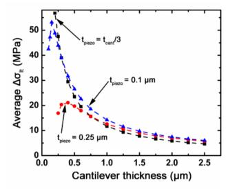
The above figure compares the piezoresistor thickness of 0.1 and  $0.25\mu m$  and the one in which the piezoresistior thickness is one third of the cantilever thickness. The relationship is inversely proportional.
