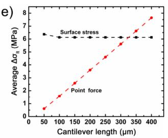
The stress difference with surface stress loading on the top surface with width  $50\mu m$  and length 200,100, 50 and  $400\mu m$  and the graph of average stress and cantilever width is shown below.
