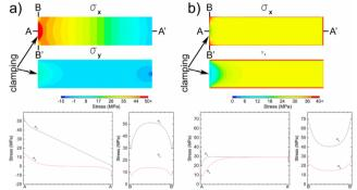
The two loading cases comparison clearly displays that the stress distributions within the cantilever and thus the piezoresistive output signal are very dissimilar. While the point force causes a stress distribution with a linearly decreasing stress in x-direction and a stress of much smaller magnitude in y-direction, this is not the case for the cantilever surface stress loading.
