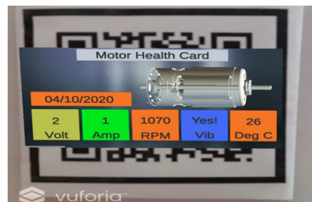
Fig. 7. Augmented Reality Projection of Motor health card.
