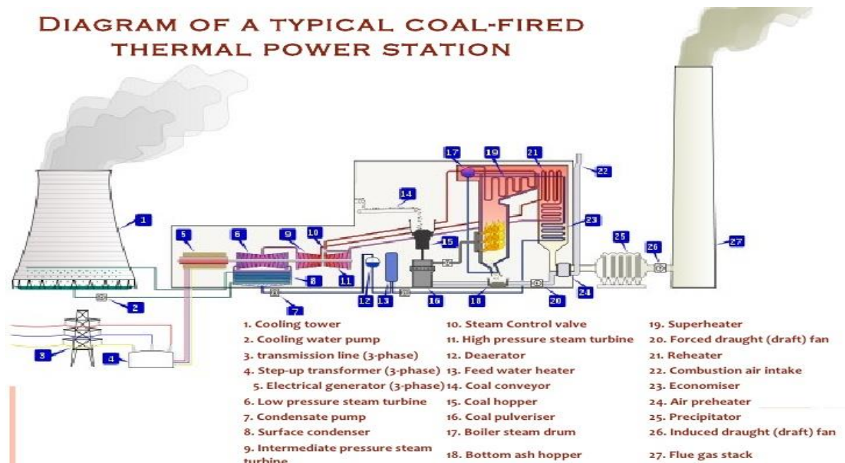
Fig 1 : Typical Coal Fired Power Plant
