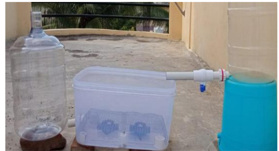
Fig No. 4. Inlet and outlet arrangements
