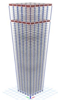
Fig. 2. Model with outriggers at H (top) and 7H/8
