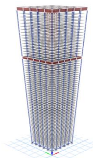
Fig. 3. Model with outriggers at H (top) and 3H/4
