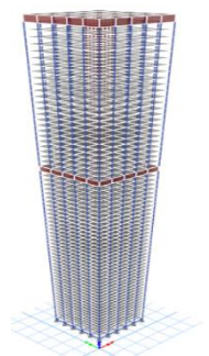
Fig. 4. Model with outriggers at H (top) and 5H/8
