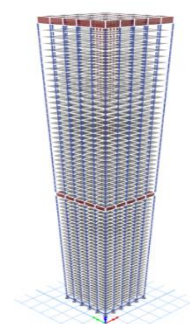
Fig. 5. Model with outriggers at H (top) and H/2
