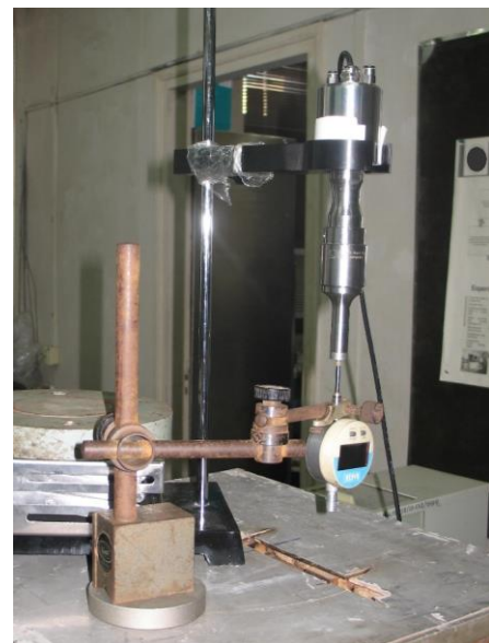
Fig. 3. Calibration by Digital Dial Indicator
