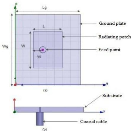
Fig. 1. Geometry of coaxial feed microstrip patch antenna [15]
