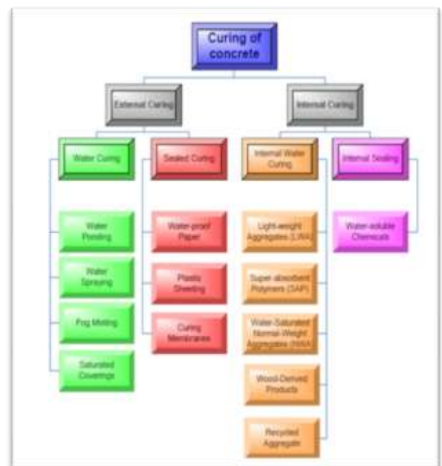
Fig 1: Different methods of external and internal curing
