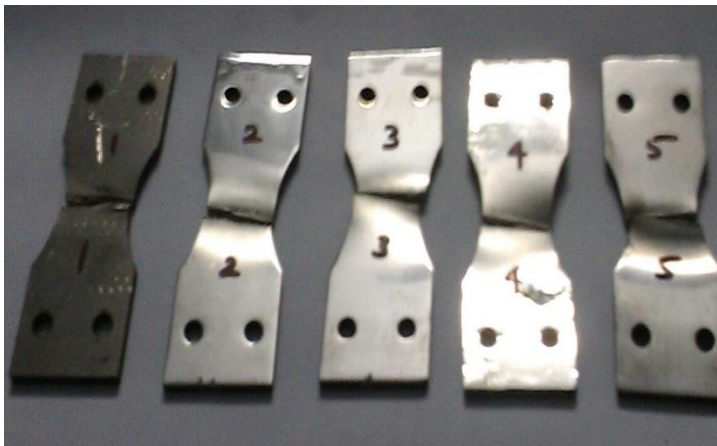
Fig 12 Specimens after bending fatigue testing
