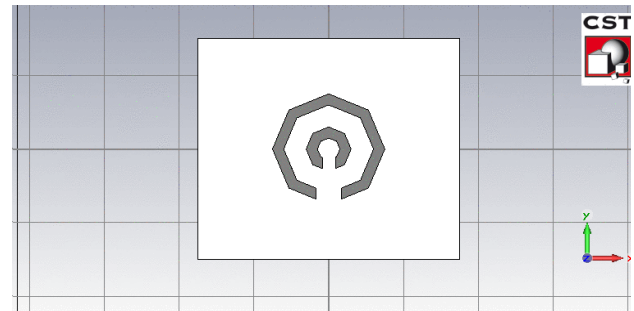
Fig. 6. Proposed design of metamaterial
