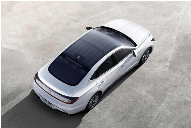
Fig. 1. Hyundai Sonata Hybrid with solar-panel roof.
