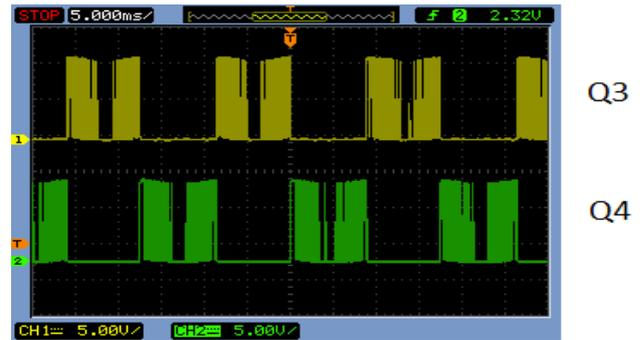
Fig. 11. Gate pulses of Switches (a) Q3 and Q4
