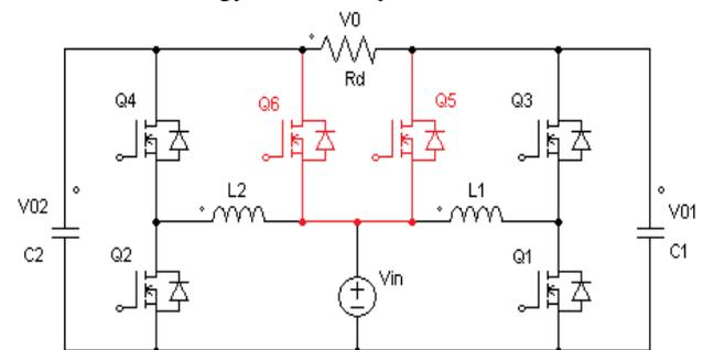
Fig. 5. Improved main circuit with clamping switches
