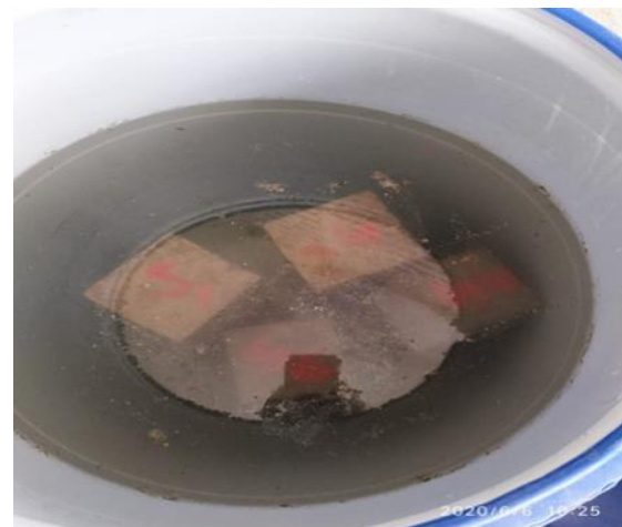
Figure.3 Cubes cured in Acid
