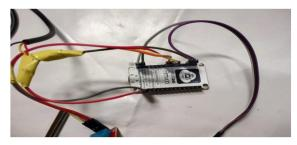
Node mcu is an open-source firmware and development kit that helps you to prototype or build IoT product. Node mcu too like Arduino Uno can be programmed directly using Arduino IDE. Node mcu has 10 digital pins and only one analog pin. Communication Interface: The user must connect to the system using Node mcu that is to gain control and a dashboard to display the results will be made currently we will be using through wifi module of the Node mcu.
