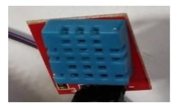
DHT temperature & humidity sensors: The low cost DHT temperature & humidity sensors. These sensors are very basic and slow, but are great for hobbyists who want to do some basic data logging. The DHT sensors are made of two parts, a capacitive humidity sensor and a thermistor. There is also a very basic chip inside that does some analog to digital conversion and spits out a digital signal with the temperature
