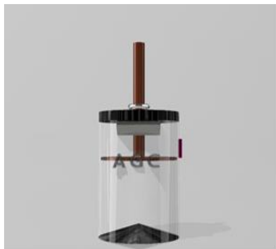
Fig. 3(b). The sensor blinks red when it gets actuated by the presence of garbage. Thus, the piston moves to the forward end position.
