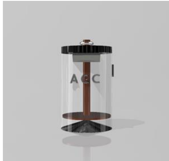
Fig. 3(c). The Piston compresses the garbage for 30 seconds and the sensor resets, retracting the piston.
