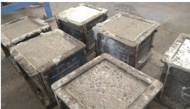
Fig -1 : Casting of Concrete blocks
