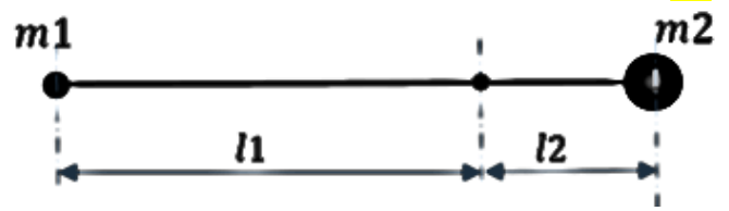
Fig.3 – Connecting rod in Two mass equivalent system.
