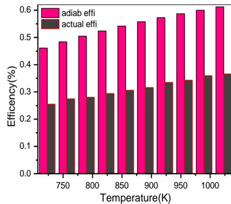
Fig. 3 Relationship between hot source temperature and engine efficiency
