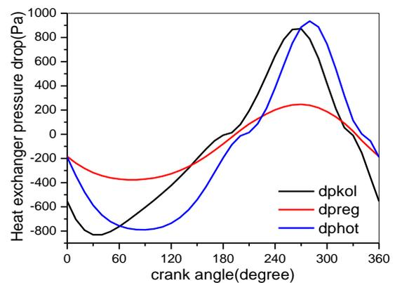
Fig. 17 Heat exchanger pressure drops virus crank angle
