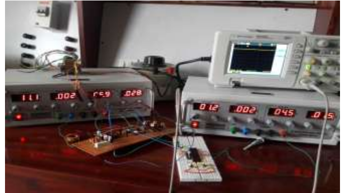
Fig. 25. Experimental setup for new transformerless buck-boost converter
